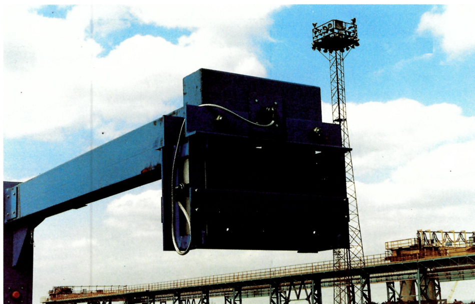
Radiation detector operating at the entry weighbridge
